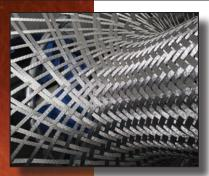
Hose Master's stainless steel wire braid gives corrugated hose the ability to withstand pressure. For increased safety, Hose Master machines the braid directly onto the hose, ensuring that the braid fits tightly against the hose to prevent the potential for hose deformation or squirm. Hose Master offers the highest percentage of braid coverage (90%) yielding better cycle life and protection against damage to the hose.
