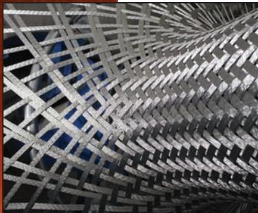
Hose Master's stainless steel wire braid gives corrugated hose the ability to withstand pressure. For increased safety, Hose Master machines the braid directly onto the hose, ensuring that the braid fits tightly against the hose to prevent the potential for hose deformation or squirm. Hose Master offers the highest percentage of braid coverage (90%) yielding better cycle life and protection against damage to the hose.
